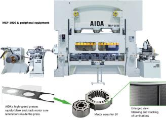
MSP-3000 High-Speed Precision Press and Peripheral Equipment
